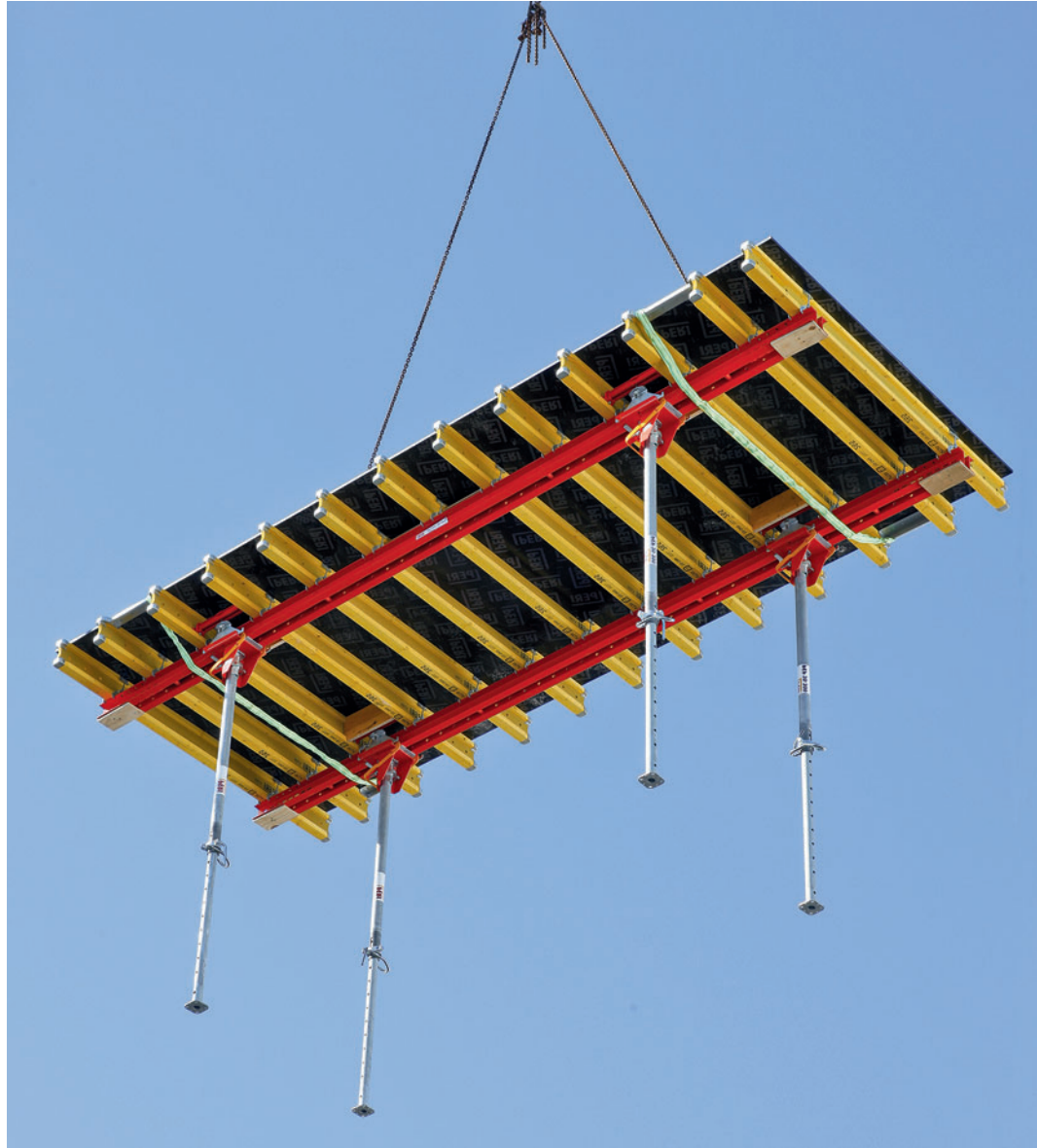
VARIODECK steel waler slab table with dimensions of 2.50/2.65 x 6.00 m requires only 4 slab props. This corresponds to a maximum 4 m 2 of slab per prop.
